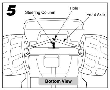
• Fit the curved end of the steering column into the hole in the front axle.
